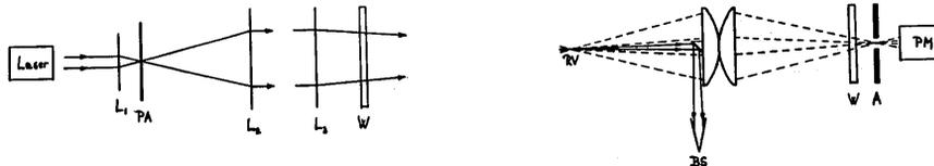
Figure 11. Schematic representation of the optical system to be used for measuring the density of microparticle targets (see text for details).
