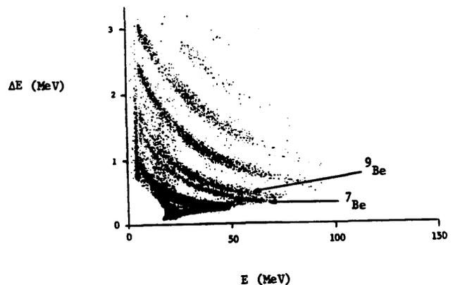
Figure 3. Point plot of  $\Delta E$  vs  $E$  at  $30^\circ$ .  $\Delta E$  obtained from shaping electrode design ionization chamber.  $E$  is a 300  $\mu\text{m}$  Si detector showing Be punch through.
