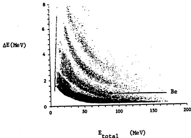
Figure 2. Point plot of  $\Delta E$  vs  $E_{\text{total}}$  at  $30^\circ$ .  $\Delta E$  obtained from multi-anode design ionization chamber.
