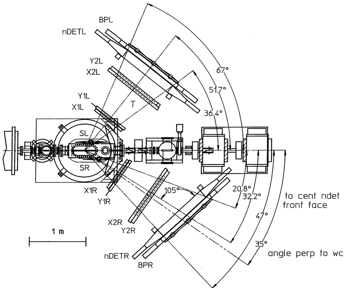
*Figure 1.* Schematic top view of the experimental setup. Protons are detected by a start scintillator (S#), two pair of x-y wire chambers (X#,Y#), a plastic scintillator array (nDET#) and additional backing plastics (BP#). Neutrons are detected only in the plastic scintillator array.
