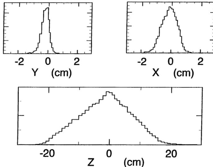
*Figure 2.* Reconstruction of the vertex position from wire chamber raytracing of two protons. The coordinate y is vertical and z is along the beam axis.
